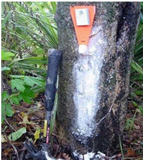
Photo 1: Waxtag monitoring device as set in the field, the green square is luminous to attract possum attention at night.
